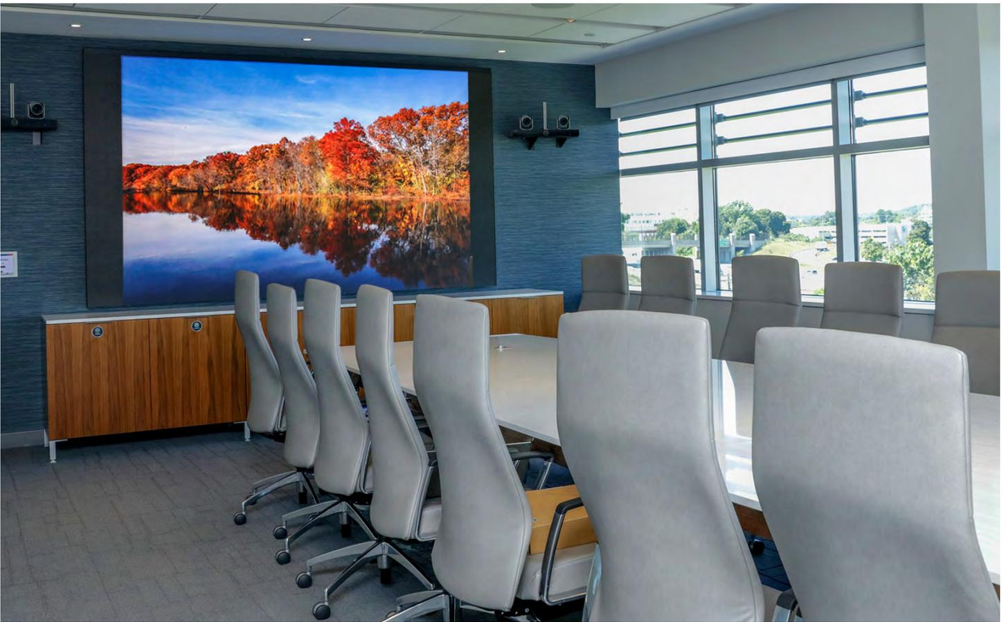
Ultimately, Fraine and the bank team selected LED display technology from Planar, leading to the installation of a nearly 10-foot-long, 6-foot-high Planar® TVF Series LED video wall with a 1.5mm pixel pitch (TVF1.5) in a 5x5 configuration—the focal point of a boardroom technology package that includes video conferencing, camera voice tracking system, retractable table microphones and wireless presentation capability.
