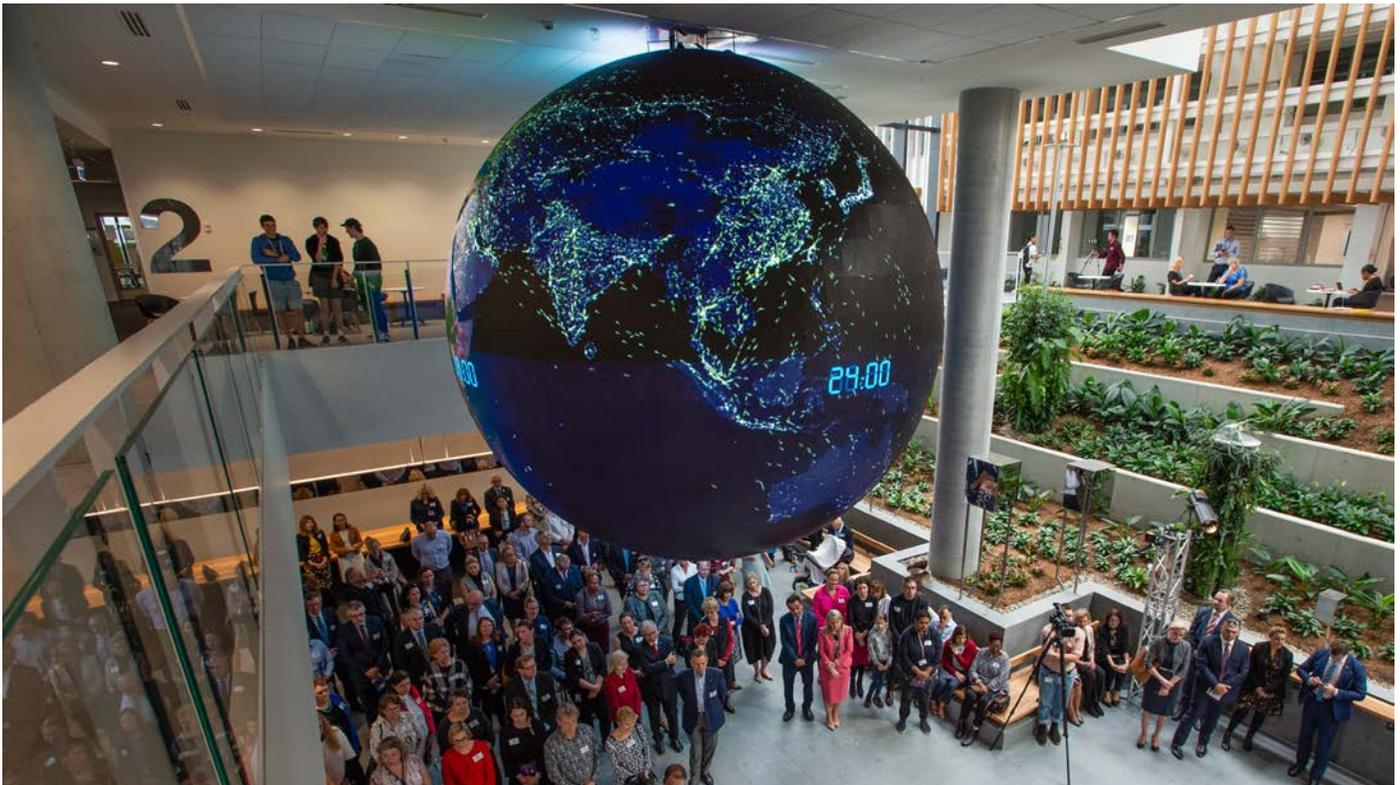
Suspended over two floors in a large, open atrium is the center attraction of the new precinct building—a massive five-meter diameter LED globe weighing 3.5 tons and composed of 1,040 individual panels and 12.7 million individual LED lights (12.7 million 3mm pixels). Built by Linso, a Leyard company, the Sphere is a first-of-its-kind digital marvel and cutting-edge research tool for the Faculty of Education to advance teacher training.
